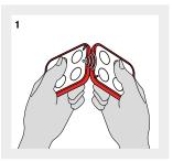
1. Exchange of identity code between a previously memorised transmitter with LoRa® technology and a new transmitter to be memorised.
