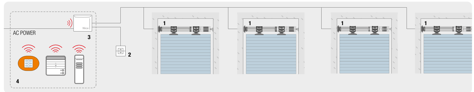
1. TUBULAR MOTOR 2. GROUP "UP/DOWN" BUTTON 3. MINDY TT4* SERIES "UP/DOWN" CONTROL UNIT 4. TRANSMITTER FOR GROUP CONTROL
